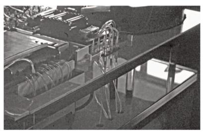
In-house assembled AutoAnalyzer, partial view of pumps and manifold
