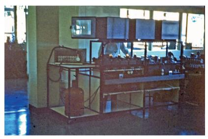
In-house assembled AutoAnalyzer, rear view
