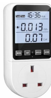
Plug-in power meter. These devices are simple to operate and can be cheaply purchased from popular online marketplaces.
