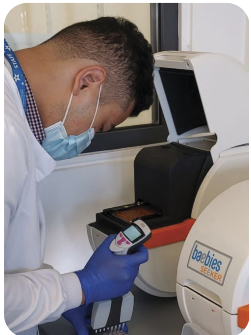
Setting up a digital microfluidics assay to measure enzyme activity in dried blood spots
