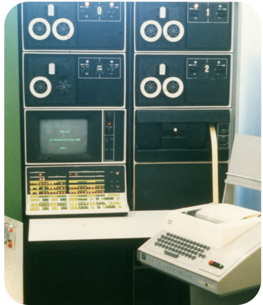
PDP 12 computer which served Northwick Park Clinical Chemistry from 1971-1984. Note random access tape memory and punched tape output
